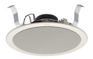
Integrated with a speaker unit and panel, the PC-2852 Ceiling Mount Speaker is of all metallic construction and ideal for use in a voice alarm system. It feature spring clamp mechanism for easy speaker mounting to the ceiling. The input impedance can be easily changed by changing the tap position of the transformer. The push-in type input terminal block makes cable connections easy and allows bridge wiring.
