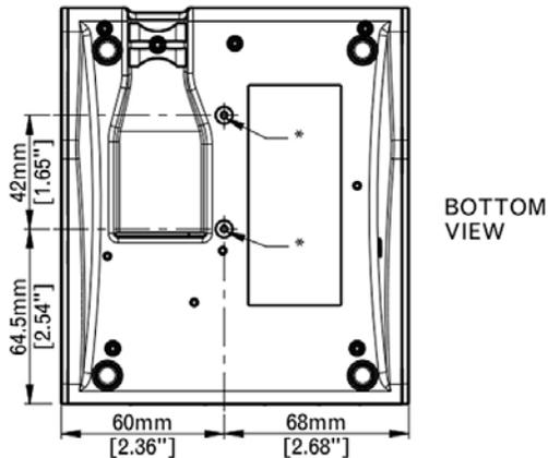
\* Drill blind hole  $\varnothing$  2.5mm, maximum depth = 6 mm for M3 thread cut.(bottom tap)
