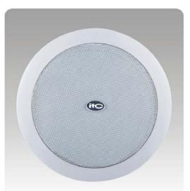
The built-in 8"+1.5" coaxial plastic speaker driver is designed of wide frequency response 60-20kHz, the multiple power taps 3.75W, 7.5W, 15W & 30W are helpful for different applications varies from room size and ambient noise surroundings. The metal grille and ABS baffle are painted in attractive white color. Its flush mount type makes the easy and secure installation.
